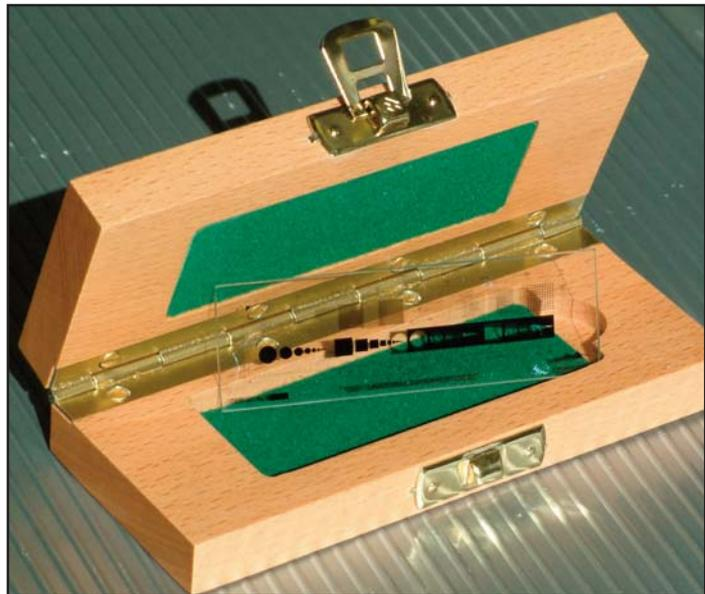
Each glass slide has a unique permanent serial number and can be supplied with full or partial UKAS certificate of accuracy.
